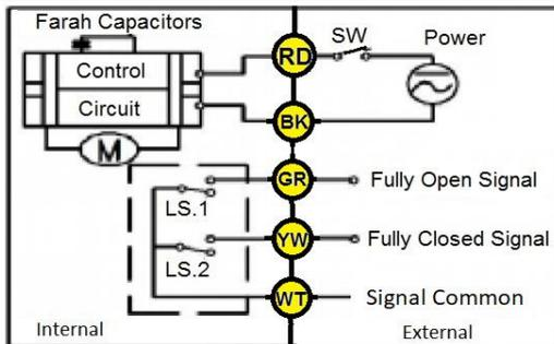
Power ON motor actuates valve into powered position and then automatically powers off. Valve stays in powered position.
