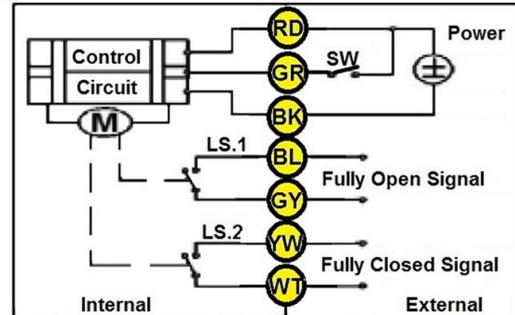
Power ON to GREEN motor actuates valve into powered position and then automatically powers off. Valve stays in powered position.
